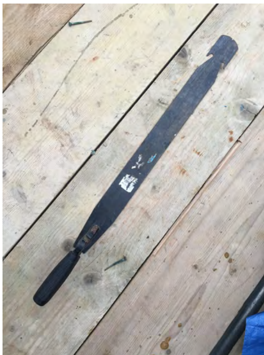
Photo 17 – Swithland slate tile removing tool, note the nails lying on the boards by the tool
