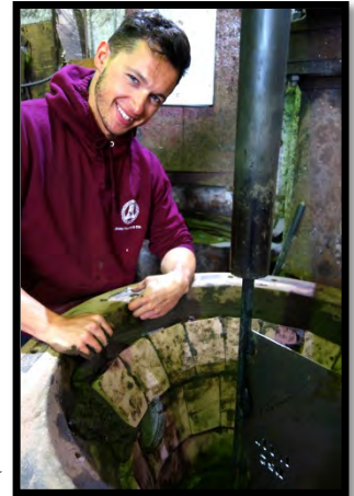
Figure 12(b). Lining the inside of the casing.
