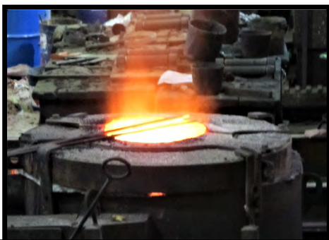
Figure 6. Heating the bronze in the furnace.
