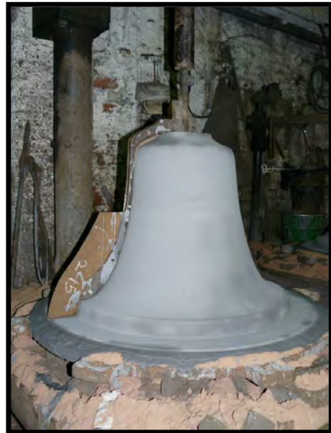
Figure 14. The inner mould (courtesy of the John Taylor Bell Foundry).
