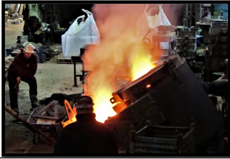
Figure 7. Pouring molten bronze into the ladle.
